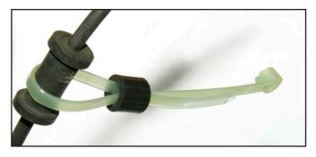
14. Secure the ABS wire to the Brake hose.
