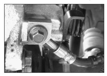
6. Remove the OEM brake hose by unbolting the mounting bracket from the frame rail.
