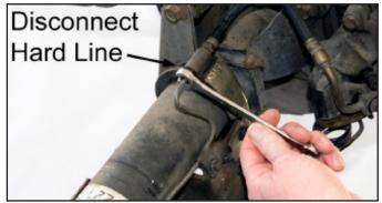
NOTE: Use a plug to cap off the hard line to prevent brake fluid loss.
