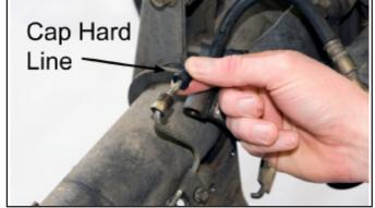
5. Remove factory brake hose/bracket assembly from the car. First, remove the screw securing the mounting bracket on the axle. This requires a Torx T-40 bit..
