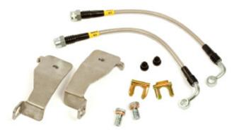
Maximum Motorsports DOT approved braided stainless steel brake hoses provide better performance because their Teflon lining does not expand under pressur like a typical rubber line will. Stainless steel hoses will provide quicker braking response, improved modulation, and a firmer brake pedal.
