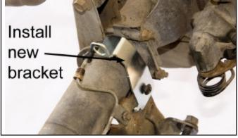
NOTE: There is a Driver and Passenger Side Brake Hose Mounting Bracket.
